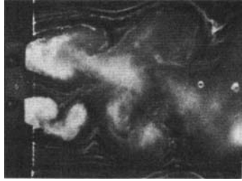
FIGURE 22. Unstable biasing of a gap flow for a two-plate row with s/d = 1.75 .
